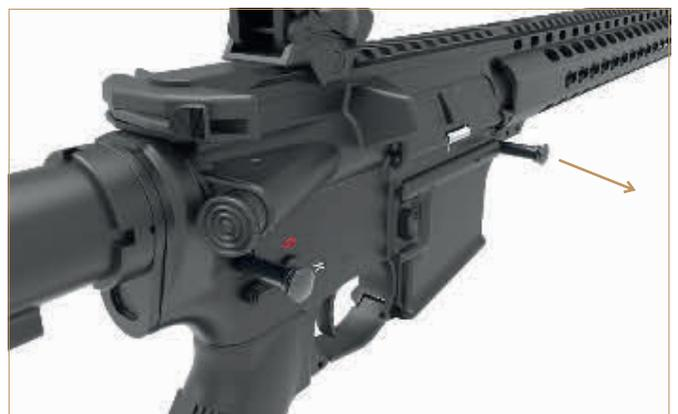
3. Remove the upper receiver from the lower receiver
