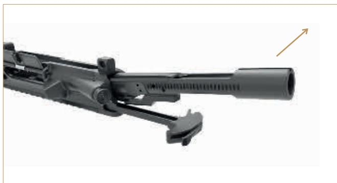
3. Pull back the charging handle up to the recess in the upper receiver and remove it upwards.
