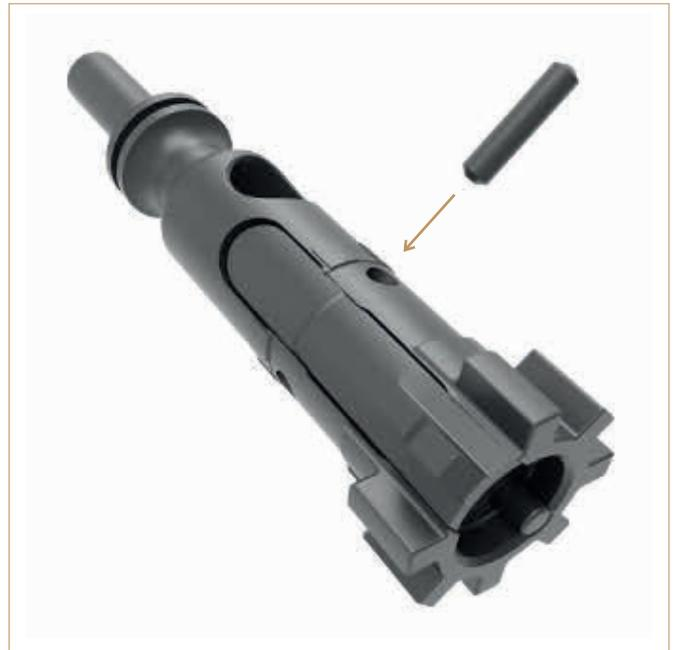
3. Insert the bolt head into the bolt head carrier so that the extractor claw is pointing at 10 o'clock
