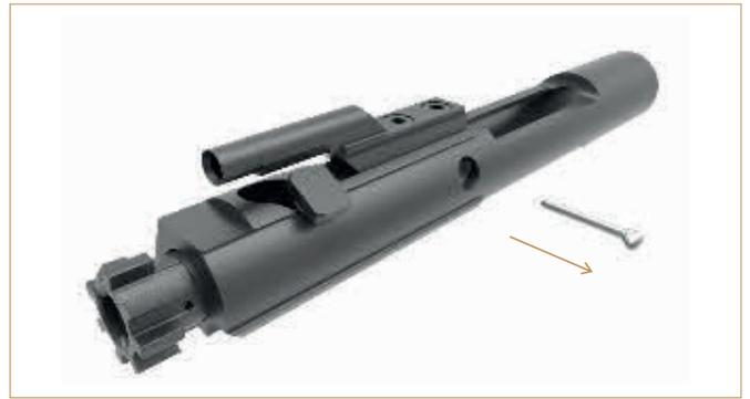
3. Guide the firing pin backwards from the bolt head carrier and remove downwards
