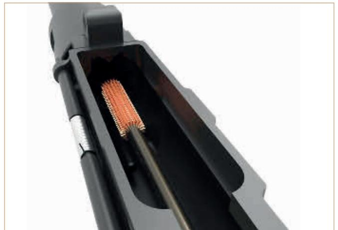
3. Remove smoke residue from locking lugs with the brush
