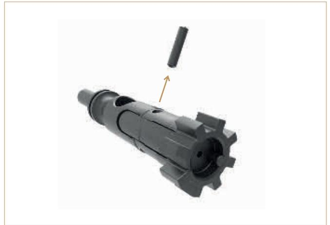
2. Remove extractor claw (make sure that you do not separate the extractor claw spring from the extractor)
