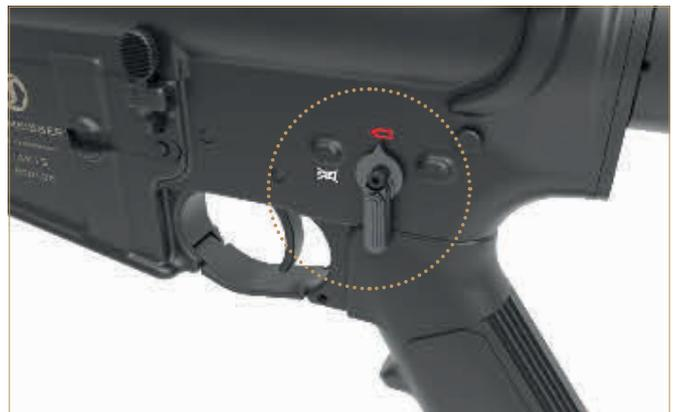
4. Hold the trigger down and cock the weapon using the charging handle at the same time; the disconnecter will hold the striker in the rearward position
