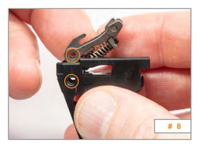
Insert the sear holder pin and ensure that it is flush with the trigger mechanism housing. (#9)
