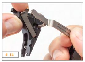
Push down on the trigger spring assembly making sure that the trigger spring rod engages with the slave pin. Then take the trigger bar and with the lower extension push out the slave pin while simultaneously guiding the top extension of the trigger bar into the recess of the trigger mechanism housing. (# 14)
