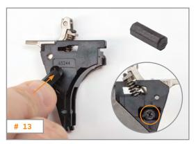
The tool shown can be used for easier installation. (# 252) Use the tool as a slave pin by inserting it from the left side of the trigger mechanism housing. (# 13)
