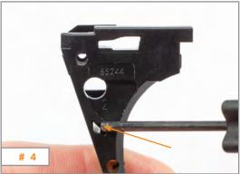
Remove the connector by pushing the GLOCK tool all the way through the hole provided on the opposite side of the trigger mechanism housing. (# 4)
