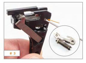
Remove the sear-holder pin by pushing it out of the trigger mechanism housing by using a 1.5 pin punch or a paperclip. The trigger spring should fall out easily. (# 3)
