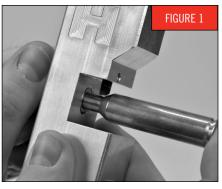
cutting bit will run down the length of the case neck by threading the mandrel in or out. This depth is ultimately up to the individual reloader, but a general guideline is to cut until the bit just makes contact with the cartridge shoulder (FIGURE 1).
