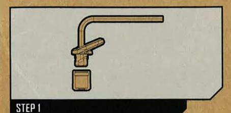
Using a 9/64" hex wrench, make sure the Paraclip Adapter Clamp Screw is loosened enough to allow the Paraclip Adapter Clamp to slide completely open.
