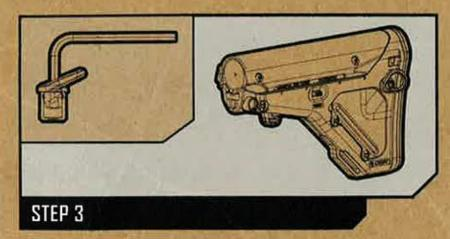
Hand tighten the Clamp Screw using a 9/64" hex wrench. Support the Paraclip Adapter Loop to prevent it from rotating as the screw is tightened.
